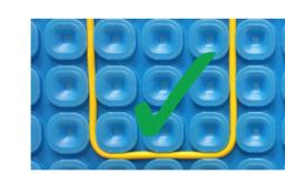
Correct heating cable spacing Heating cables should be installed in runs spaced between every second (195W/m<sup>2</sup>) or third (130W/m<sup>2</sup>) m<sup>2</sup>) row. The heating cables should never cross.
