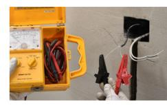
4. Complete the testing procedure After laying the tiles, repeat all of the tests and record the values to allow the end user to register their warranty online at www.thermosphere.com.
